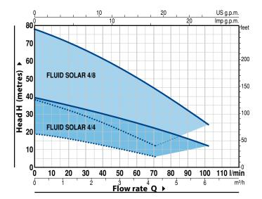
Tolerance of characteristic curves in compliance with EN ISO 9906 Grade 3B
