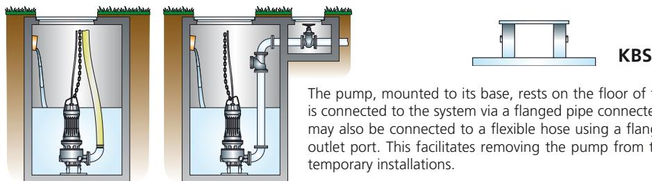
The pump, mounted to its base, rests on the floor of the tank in the vertical position. It is connected to the system via a flanged pipe connected to its discharge port. The pump may also be connected to a flexible hose using a flanged bend union connected to the outlet port. This facilitates removing the pump from the tank and is recommended for temporary installations.
