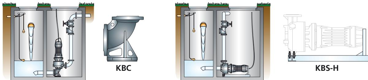
The pump may be installed in a dry chamber by using a cooling jacket.
