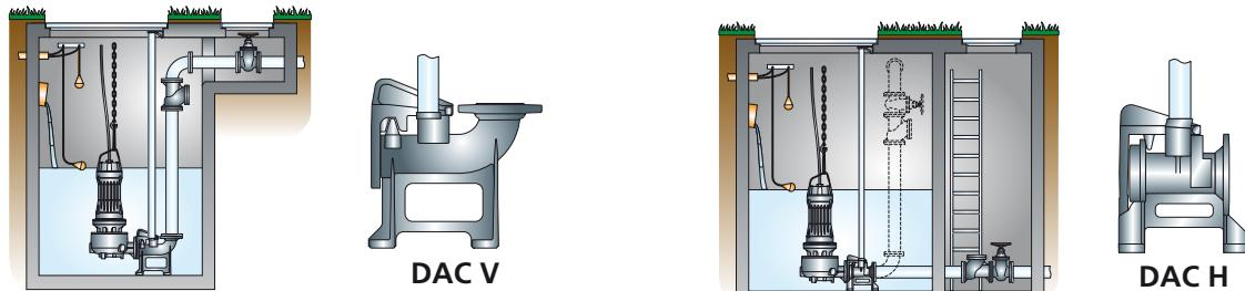
The vertical or horizontal coupling device is fixed to the bottom of the tank and the pump is lowered in with the aid of two guide pipes fitted earlier, until the connection to the foot is completed.
