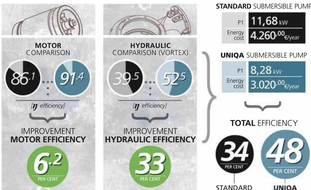
The example highlights the fact that using a **UNIQA pump with efficiency class PREMIUM IE3 (+6.2%) motor and high performance hydraulics (+33%) compared to a STANDARD pump, yields improved global system efficiency, at the duty point in question, of 6%, thus providing considerable cost savings.**
